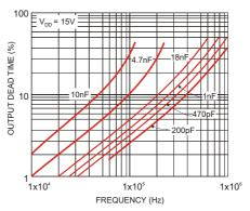
Figure 2. GM38C42, GM38C43 Output Dead Time vs. Oscillator Frequency
