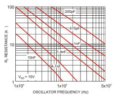
Figure 1. Oscillator Frequency Configuration
