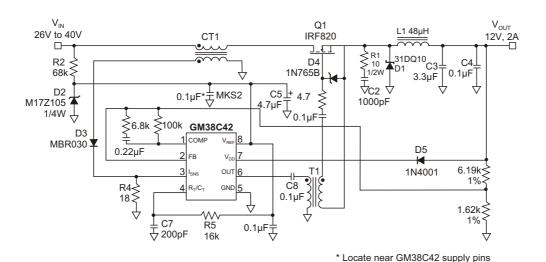
Figure 7. 500kHz, 25W, Buck Converter
