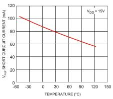
Figure 5. Short - Circuit Reference Current vs. Temperature
