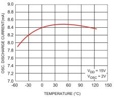
Figure 3. Oscillator Discharge Current vs.
