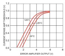
Figure 4. Current Sense Amplifier vs. Error Amplifier Output
