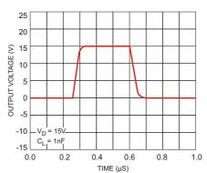
Figure 6. GM38C4X Output Waveform
